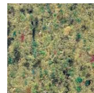
2,5 mm linoleum + 1,5 mm recycled foam
